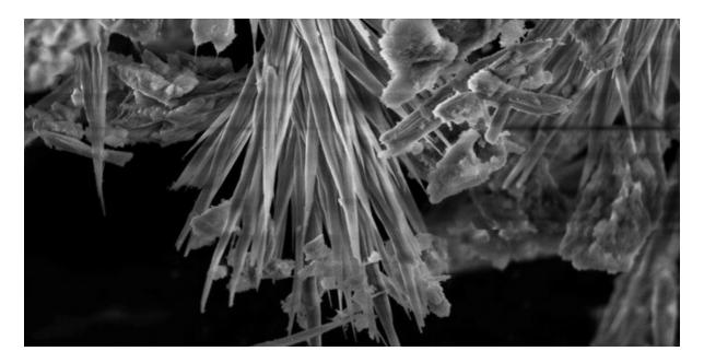
These nanocrystal spikes, formed from nickel and iron, can convert water into oxygen and hydrogen. Rutgers chemist Kate Waldie is studying these and other new materials to improve the efficiency of producing hydrogen fuel using renewable energy.
